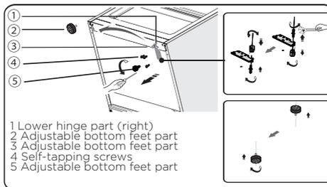
12. Remove part 3 from the lower hinge pin, loose out the lower hinge pin, change it to the reverse hole site, and then tighten into position, then install part 3 on the lower hinge pin.
