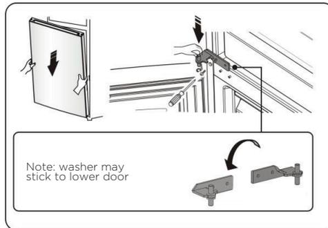
15. Move the upper door to an appropriate position, and then fix part 2 by screws 1. Before fix part 2, pass connector 3 through hinge 2 refer to step 3. (Please hold upper door by hand when installing).
