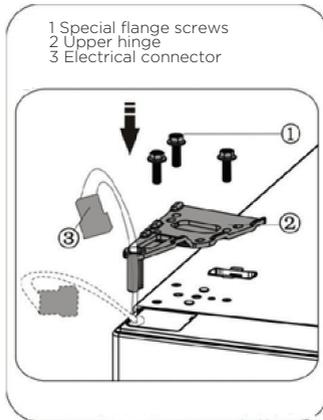
16. Connect electrical connector 1 as shown in the picture, then fix part 2 by screw 3 refer to step 2.
