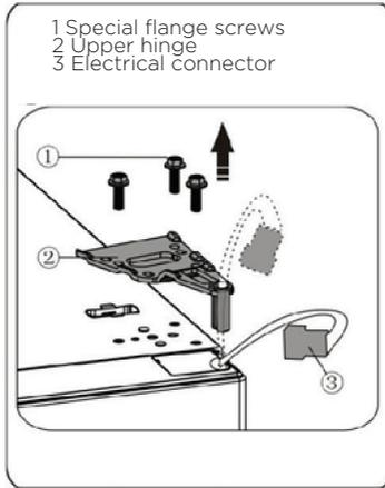
4. Remove the upper door from the middle hinge by carefully lifting the door straight up. Then place the upper door on a smooth surface with its upper cover upwards.
