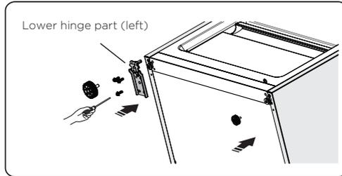
14. Slot the lower door onto the bottom hinge pin and hold in position. Turn the middle hinge by 180°, change the washer on the axis to the lower side, adjust the middle hinge to the appropriate position and then install it ensuring the lower door is secured in place.
