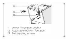
11. Replace the lower hinge part to the left side and fixing it with the special flange self-tapping screws. Replace the adjustable bottom feet parts to another side and fixing it.
