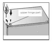
16.Install the screw hole cover on the top right corner of the refrigerator. Install the upper hinge cover (which is in the plastic bag) on the left corner. Put the other upper hinge cover into the plastic bag.
