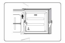
6. Place the upper door on a smooth surface with its panel upwards. Loose screw (2) and part (1), then install them to the left side and tighten securely.
