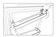
Press the right side of the door shelf inwardly ,while holding the left side . When the notch of the shelf has been detachesd from the refrigerator door , remove the rack obliquely upwardly.
