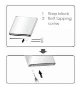
7. Unscrew the two special flange self-tapping screws which are used for fixing the middle hinge part, then remove the middle hinge part that hold the lower door in place.
