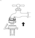
Connect the inlet hose adapt. of the hose to the water inlet of the washer by turning it clockwise to be fixed tightly.
