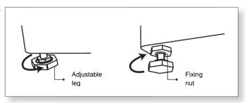
Make it sure that the washer does not sway when you press down the four corners of the washer's top plate.
