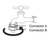
Connect the inlet hose to the water tap adapter by pulling down the collar of the hose end
