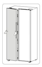
5. Remove all shelves and drawers inside the appliance. Tip the refrigerator backwards, remove the screws fixed on the hinge with a Wrench. Then remove the lower hinge.
