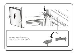
15. Move the upper door to an appropriate position, and then fix part 2 by screws
