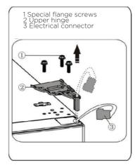
4. Remove the upper door from the middle hinge by carefully lifting the door straight up. Then place the upper door on a smooth surface with its upper cover upwards.
