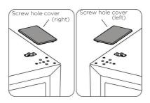
6. Remove part 1 from the top left side of upper cover and take out part 2. Then remove part 3 from the top right side of upper cover. Refer to above operation, install part 3 and part 4 onto the top left side of upper cover. Install part 1 of the top right side of upper cover.
