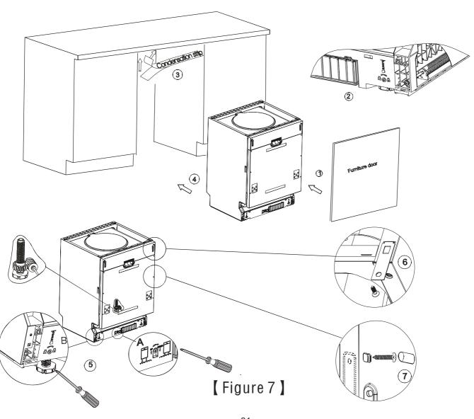
Dishwasher must be level for proper dish rack operation and wash performance.
