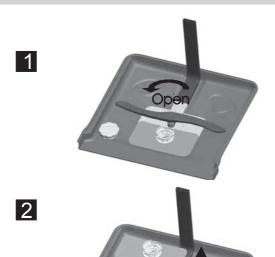
Step 1: Turn the filter in anti-clockwise direction,
