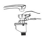
The appliance must be connected to the water mains using new hose-sets. The old hose-sets should not be reused.
