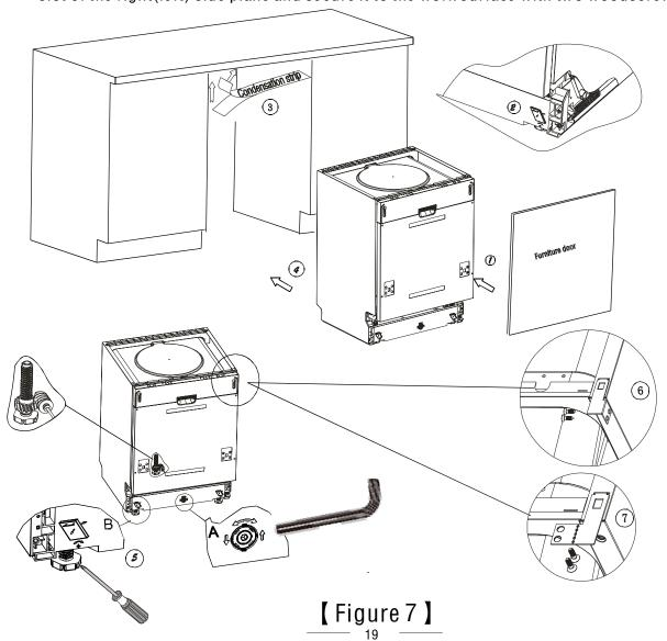
Dishwasher must be level for proper dish rack operation and wash performance.
