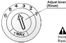
The rinse aid dispenser has six or four settings. Always start with the dispenser set on "4". If spots and poor drying are a problem, increase the amount of rinse aid dispensed by removing the dispenser lid and rotating the dial to "5". If the dishes still are not drying properly or are show spots, adjust the dial to the next higher lever until your dishes are spot-free. The recommended setting is "4". (Factory value is "4".)
