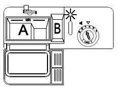
If the dishes are heavily soiled, place an additional detergent dose in the pre-wash detergent chamber. This detergent will take effect during the pre-wash phase.
