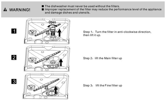
**NOTE:** When following this procedure from step1 to step 3, the filter system will be removed; when following it from Step 3 to Step 1, the filter system will be installed.
