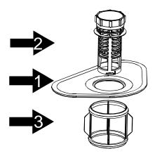
The filter system consists of a coarse filter, a flat (Main filter) And a microfilter(Fine filter).
