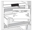
Place the appliance in a dry and well aired room. The permitted ambient temperature range for the appliance depends on the appliance's climate class, which is shown on the type plate.
