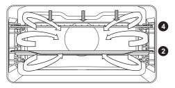
In this operating mode, the grill heater and the fan operate simultaneously. Suitable for grilling meat, fish, and vegetables.
