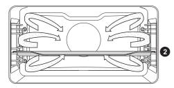
Water from the steam generator enters the oven cavity in the form of steam. In addition, round heater with fan operates to provide continuous circulation of the hot air and steam.
