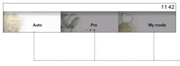
Turn the KNOB and select the name of the menu. Confirm the selection by pressing the KNOB. The NAME of the selected menu appears above.
