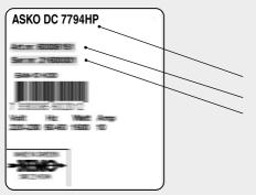
The illustration shows the identification plate for the DC7794HP drying cabinet
