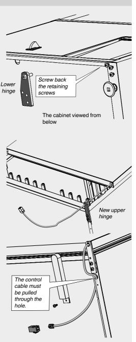
14 Transfer the hinge to the other side. The hinge must be mirror-inverted and the hinge pin must be unscrewed and refitted on the other side of the hinge.
