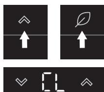
1. Simultaneously touch the adjustment key on the right and the ECO/Child Lock key for a few seconds.
