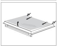
3 Slightly lift the door glass and remove it from the clips on the bottom side of the door.
