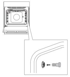
Remove the metal cap (the socket is in the front upper corner of the oven left wall).
