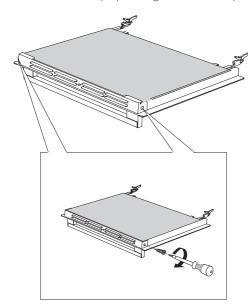
1 Undo the holder screws on both sides of the door.
