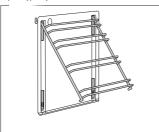
Mount the guides onto the catalytic insert.
