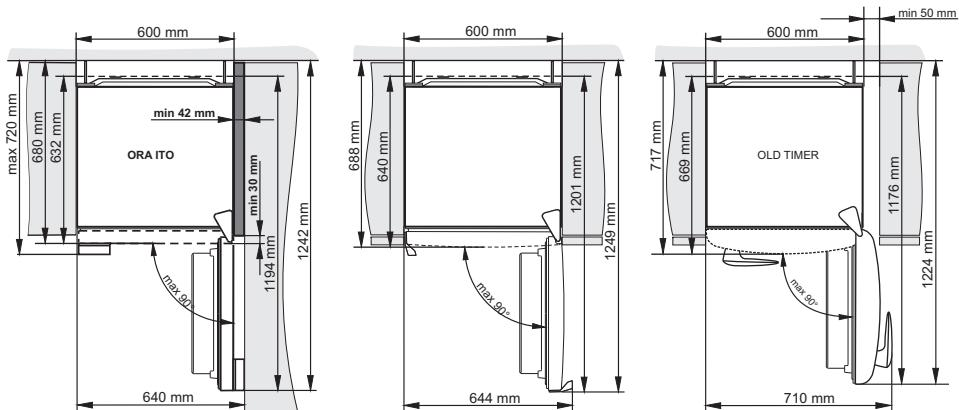
**Note:** When placing the appliances side by side, the anti-dew (anti-condensation) set has to be purchased and installed!
