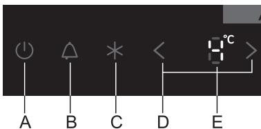
If the temperature inside the appliance is too high, acoustic alarm will be activated (**intermittent tone**) and the **B** key will flash.
