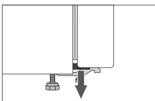
Remove the packaging intended for protecting the appliance or particular parts during transport.
