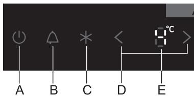
Use this function if you do not wish to manually adjust the appliance settings. To activate, press and hold the **B** key (for three seconds); **LL** will appear on the display **E**.
