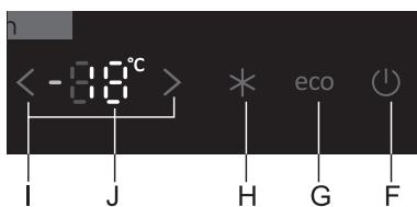
To activate the **Eco** function, press the **G** key. With this function activated, appliance will operate with optimum settings.
