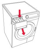
To remove the dispenser tray from the housing, press the small lever.
