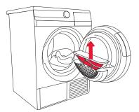
Open the filter cover, and remove the net filter.
