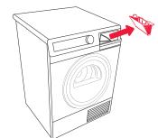
Each time you empty the condensate tank, clean the steam generator tank filter.
