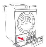
Use the handle to remove the heat pump foam filter from the dryer.
