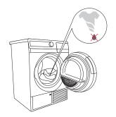
Insert wrung or spun laundry into the drum. Recommended spinning rate is at least min. 800 rpm.
