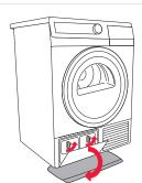
Place an absorbent cloth on the floor in front of the dryer.
