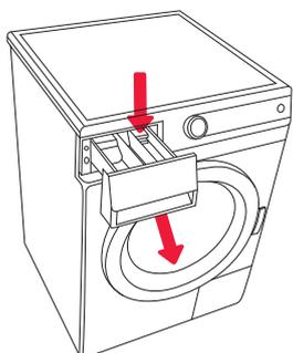
**1** To remove the dispenser tray from the housing, press the small lever.
