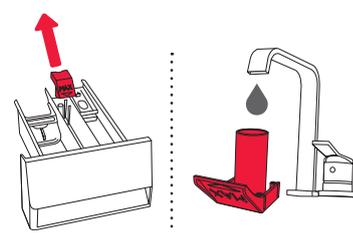
**3** If required, remove and clean the plug cap.
