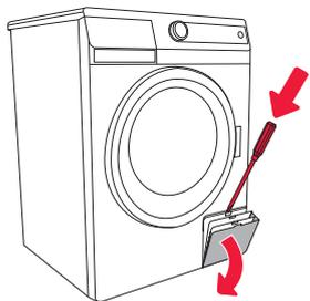
**1** Open the filter lid using flat screwdriver or similar tool.
