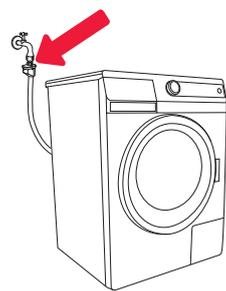
**1** Remove the net filter from the inlet hose.
