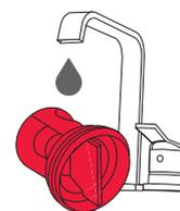
**3** Clean the filter under running water and replace it.
