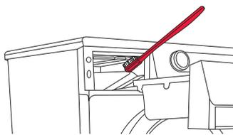
**2** In particular, clean the nozzles on the upper side of the rinsing chamber with a brush.
