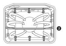
This feature allows gentle, slow, and even baking that leaves the food soft and juicy. It is suitable for roasting meat, cooking fish, and baking pastry on a single rack.
