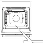
Turn the COOKING SYSTEM SELECTOR KNOB to Aqua Clean. 2. Set the TEMPERATURE KNOB to 70 °C.
