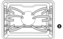
Round heater and the fan will operate. The fan installed in the back wall of the oven cavity makes sure the hot air constantly circulates around the roast or pastry.
