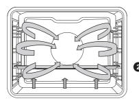
The bottom heater, the round heater, and the hot air fan will operate. Suitable for baking pizzas, apple pies, and fruitcakes.
