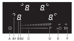
Touch the on/off sensor key (A) and hold it for at least 1 second. The cooking hob will be activated and the display units will light up.
