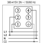
The appliance is designed for two-phase connection; it can also be connected to a single phase.
