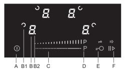
To activate the automatic rapid heating, select the desired cooking zone by touching the (B) key. Then, set the desired cooking power on the slider (C). Hold a finger on the selected level for around 3 seconds until you hear a beep and "A" appears on the display unit (B).
