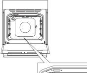
Turn the COOKING SYSTEM SELECTOR KNOB to Aqua Clean. 2. Set the TEMPERATURE KNOB to 70 °C.
