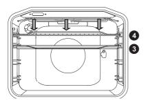
When grilling food with the large grill, the upper heater and the grill heater fitted on the ceiling of the oven cavity will operate.
