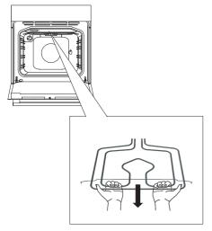
Pull the heater until the cross bar is released from the supports on the left and right hand side of the oven cavity.
