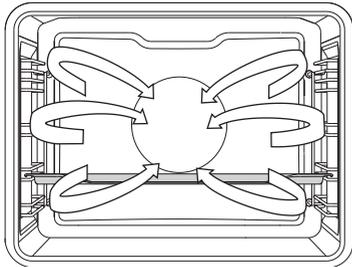
Water from the steam generator enters the oven cavity in the form of steam. In addition, round heater with fan operates to provide continuous circulation of the hot air and steam.
