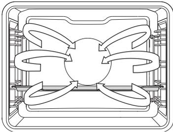
Water from the steam generator enters the oven cavity in the form of steam.
