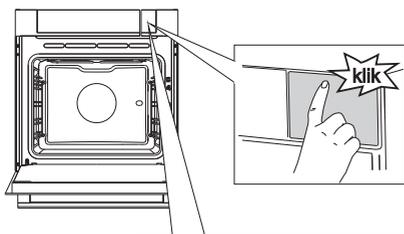
**1** Press on the spot with the sticker to open the tank door.
