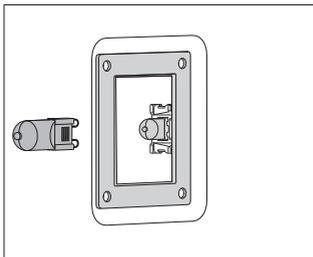
**2** Remove the halogen bulb.
