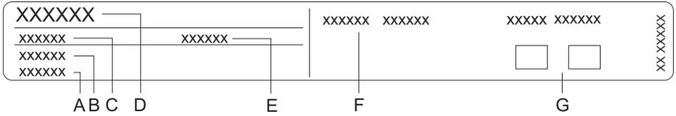
The rating plate indicating the basic information about the appliance is located at the edge of the oven and it is visible when the oven door is opened.
