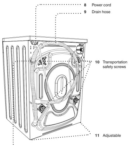
12 Drain hose holding plastic: (The operation of the machine will be affected if this plastic part is removed. So please don't remove this plastic part under any condition.)
