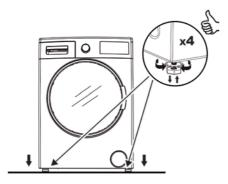
Do not install your machine on a carpet or such ground that will block ventilation from the base.
