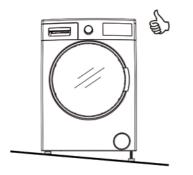
You can adjust the balance of your machine by means of the adjustable feet.
