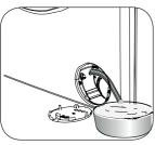
Your machine contains a filter system that prevents thread or fluff left over from your laundry and other small materials from entering the pump during the discharge operation after a completed wash cycle. This is to protect and prolong the life of the pump. It is recommended that you clean your pump filter once every 2 months.
