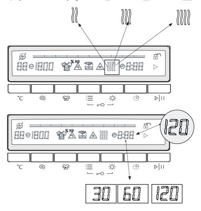
If you keep touching the button you will see the drying duration (30 min, 60 min, 120 min) options on the screen. You can select the drying duration you desire.
