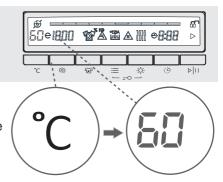
You can gradually decrease the washing water temperature between the maximum temperature and cold washing (--) by pressing the washing water temperature adjustment button.
