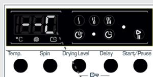
If you have missed the washing water temperature you wanted, you can return to the intended temperature by continuously pressing the washing water temperature adjustment button.
