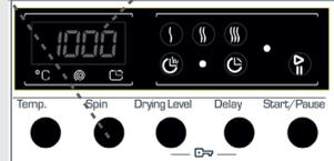
You can gradually reduce the revolution speed between cancel spinning (--) options through the maximum spin revolution of the programme selected by pressing the revolution speed setting button.
