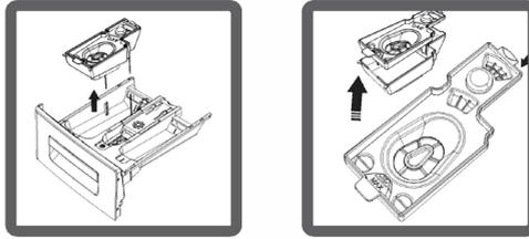
Disassemble the detergent drawer. Disassemble the siphon cover and clean the softener residues completely. Replace the siphon cover after cleaning it. Check whether it has settled properly.
