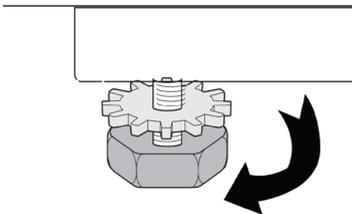
You can adjust the balance of your machine by placing a spirit level on the top. You can adjust the balance of your machine by means of the adjustable feet.
