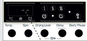
If you have skipped the spinning revolution you want to set, you can re-switch to the revolution by keeping the revolution setting button pressed.
