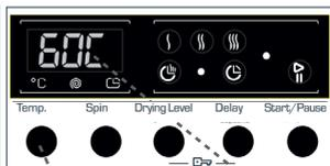
Whenever you select a new programme, the maximum washing water temperature is shown on the washing water temperature display.
