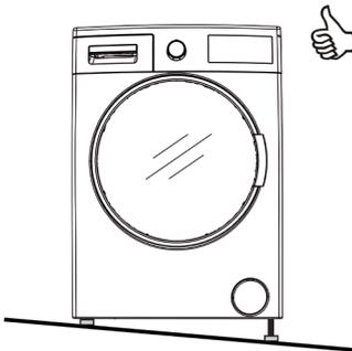
To ensure silent and vibration-free operation of your machine, it should be deployed on a non-sliding and firm ground.
