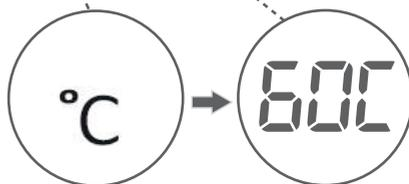
You can gradually decrease the washing water temperature between the maximum temperature and cold washing (--) by pressing the washing water temperature adjustment button.
