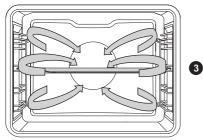
Round heater and the fan will operate. The fan installed in the back wall of the oven cavity makes sure the hot air constantly circulates around the roast or pastry.
