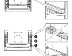
With telescopic extendible guides, first pull out the guides of one level and place the grid or the baking tray onto them. Then, push them in with your hand as far as they will go.
