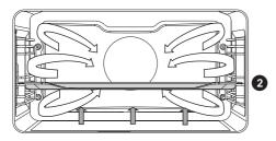
This is used for baking leavened but lowrising pastry and for preserving fruit and vegetables. Use the second guide from the bottom and a rather shallow baking tray to allow the hot air to circulate across the upper side of the dish.
