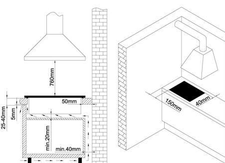
• The appliance may be built into the 25 to 40 mm thick worktops.
