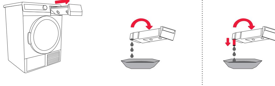
**1** Remove the condensate tank from the dryer.
