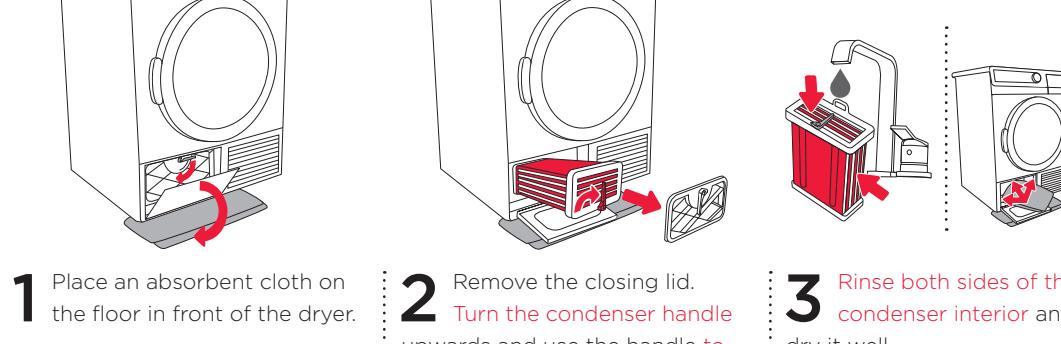
**1** Place an absorbent cloth on the floor in front of the dryer.
