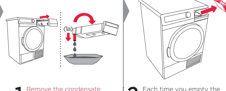
**1 Remove the condensate tank and turn it upside down above the sink or vessel to empty.**
