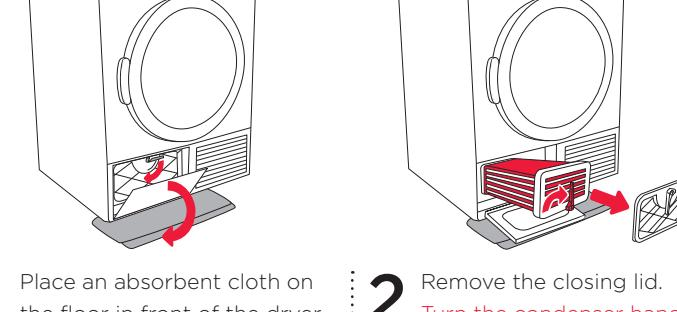
**1 Place an absorbent cloth on the floor in front of the dryer.**
