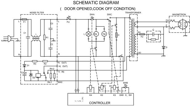
SWA: PRIMARY INTERLOCK SWITCH SWB: SECONDARY INTERLOCK SWITCH SWC: THE MONITOR INTERLOCK SWITCH
