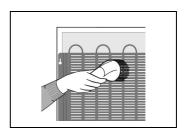
Do not forget to clean also the defrost water receptacle above the refrigerator compressor (do not remove the receptacle).
